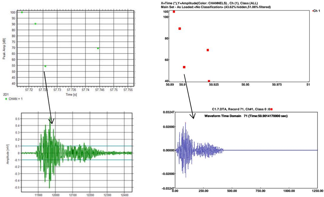
**Figure 5: Calibration of the two systems (Vallen left and Mistras right) with pencil lead breaks.**
