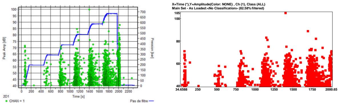
**Figure 6: AE activity during hydraulic pressure test of COPV (Vallen left and Mistras right).**
