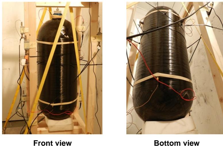
**Figure 4: An example of sensors location on 36L Hexagon COPV. (Burst chamber CEA)**
